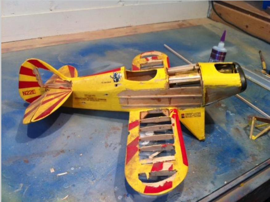
**The landing gear, struts, control system and a few other parts had to be fabricated. After finding pictures of decals on the computer we reproduce them. Time and patience was the key here, but it was successfully completed.**
