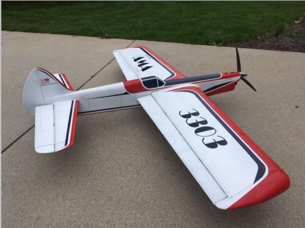
**Pictured above is my new build, the "Davis Special," designed by the late Roger Wildman. This is probably the lightest ( 61 oz.) stunt ship I've ever built. Bob Hunt lost foam wing, Tom Morris controls, carbon .02 valve, Brodak paint and powered by a Randy Smith PA 75RE.**
