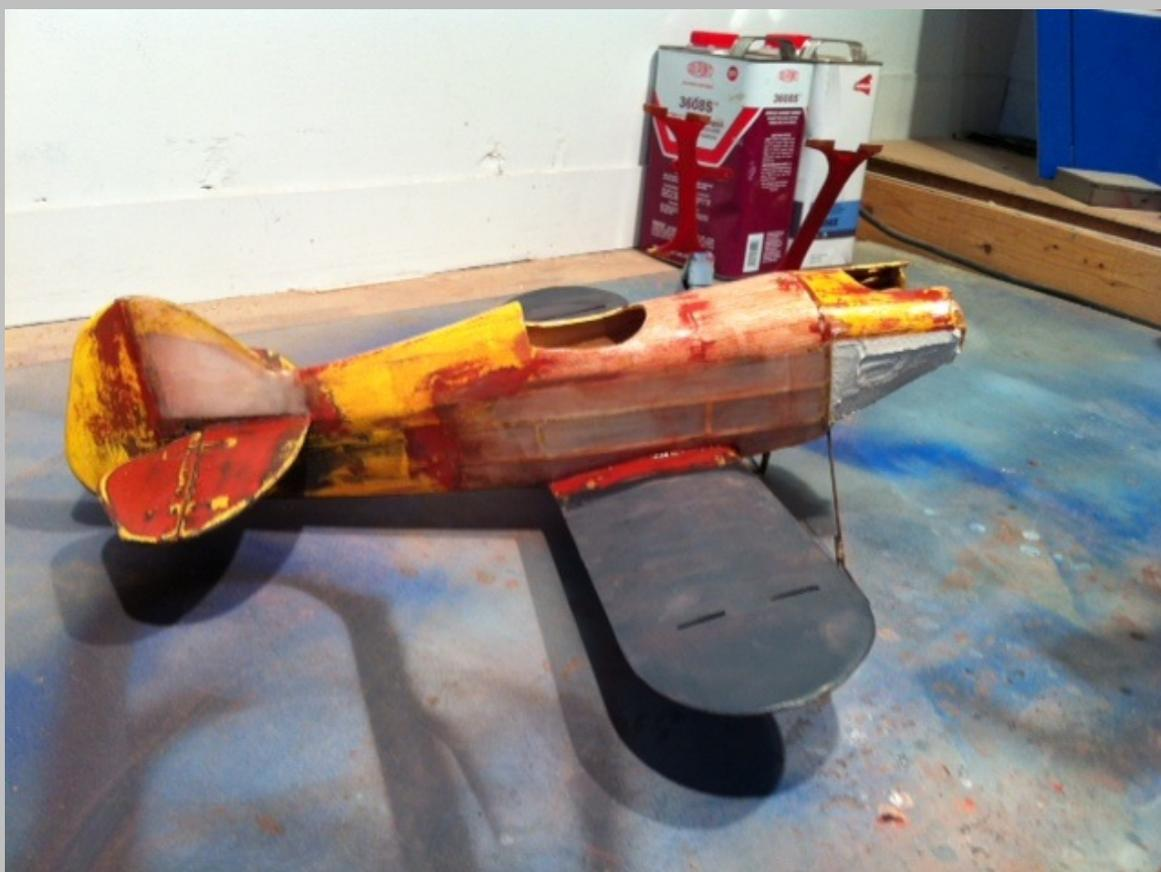
**Sanded with new covering, some fiberglass and shaping. I had some leftover Solartex from a build long ago and it worked well here.**
